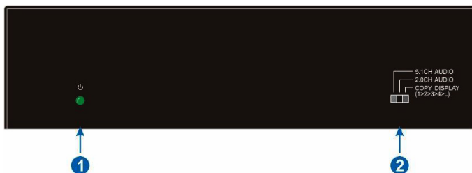
Figure 1: 1x4 HDMI 1.4 Splitter/Extender Front Panel Layout
